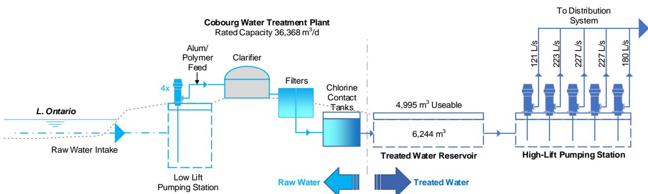
In addition to the main treatment processes above other processes and systems at the Cobourg WTP include a zebra mussel control system for the intake, a filter back-wash system, a waste handling system for disposing of wastewater and slurry from the clarifier and filters, stand-by power (generator) systems, HVAC systems as well as instrumentation for sampling water and controlling processes.
